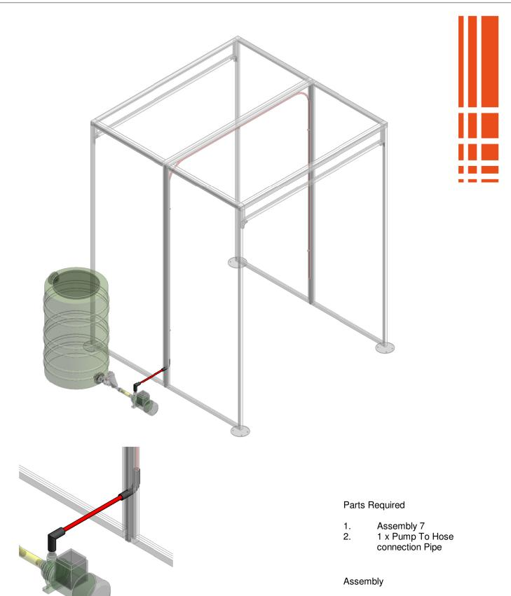
Connect Connection Pipe to Pump and Hose
